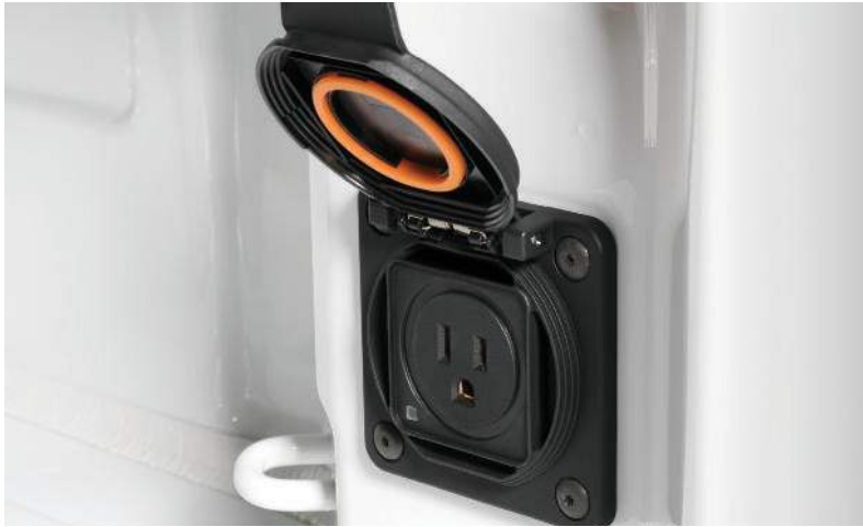
Standard 120-volt power outlet in bed
